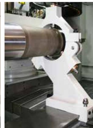
adjustment and continuous control of the force between centers with the possibility of footer pedal control.
