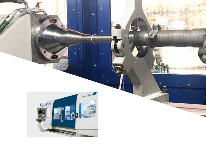
screw system and linear guideways. The workpiece is clamped by headstock and supported by steady rest moves easily on the table. Base is specifically designed to obtain the best result between structural deformations and vibration dumping. The table is realized in two cast iron parts. As optional the table can swivel CNC or manually controlled.
