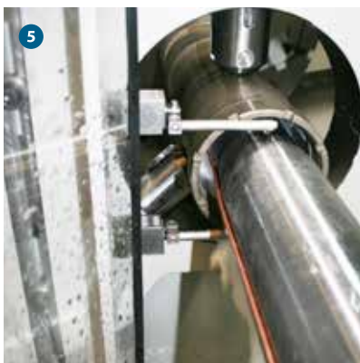
1-2. Absolute in-process measuring device 5. External measuring with double touch
